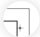
Holes in the reverse for cabinet attachment
